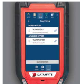
Automatically detect, display serial number, and use correct gage as characteristic's data source
