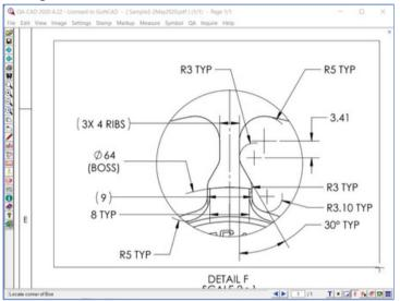
2) Then QA-CAD instantly draws automated balloons to all selected dimensions. Of course, QA-CAD extracts dimensions, tolerances, and notes at the same time. QA-CAD can balloon specific page areas or the entire page with just a few button operations.
